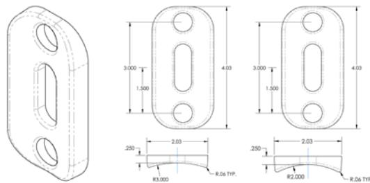
**ROUND POLE ADAPTER (RPA)** – When using round poles, specify Round Pole Adapter (RPA). Specify RPA4 when installing on 3"-4" round poles, and RPA5 when installing on 5"-6" round poles.
