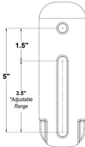
\* Elongated slotted hole to accommodate most existing pole drill patterns.
