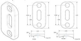
**ROUND POLE ADAPTER (RPA)** – When using round poles, specify Round Pole Adapter (RPA). Specify RPA4 when installing on 3"-4" round poles, and RPA5 when installing on 5"-6" round poles.
