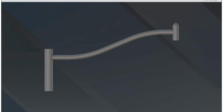
Architectural Arm 15 is constructed of extruded aluminum tubing for pendant mount luminaires. Integrates with poles or tenons of 3-1/2", 4", 4-1/2", or 5" OD and is secured with 3/8" stainless steel Allen set screws.
